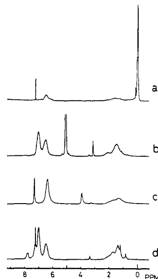
Figure 1. NMR spectra of poly(1), a; poly(aminostyrene hydrochloride), b; poly(aminostyrene), c; poly( p -vinylbenzanilide), d.
